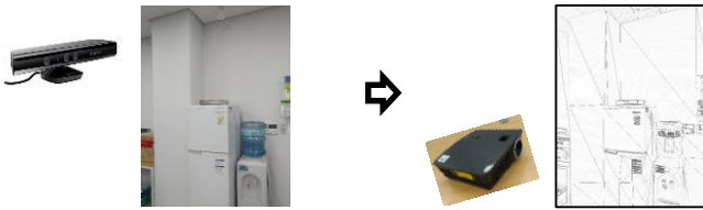
Figure 2: Screen modeling with range sensor and projection into that screen model. (Mesh model is concept image.)
